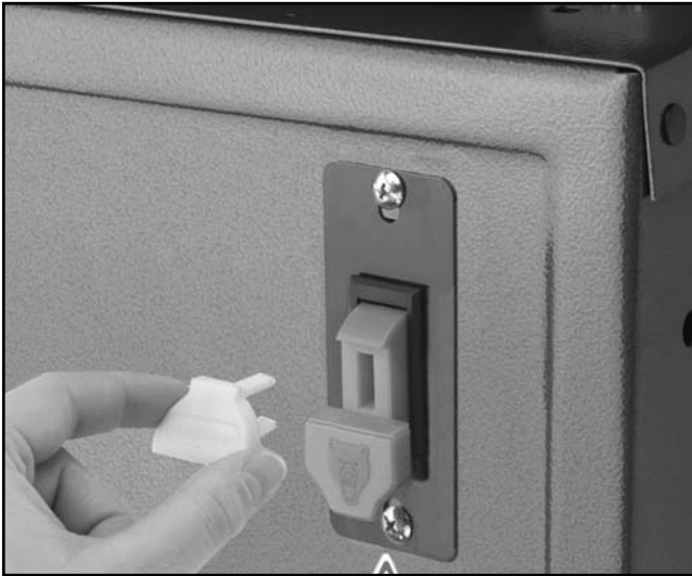
Figure 12. Removing lock-out key from switch.
